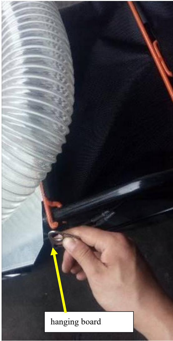
Fig.10-4 Assembly left hanging board
