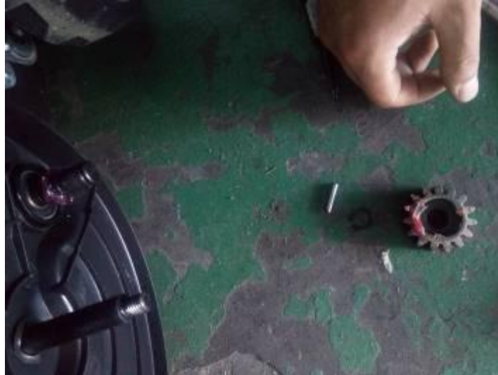
Fig.39-2 Add grease to the output shaft
